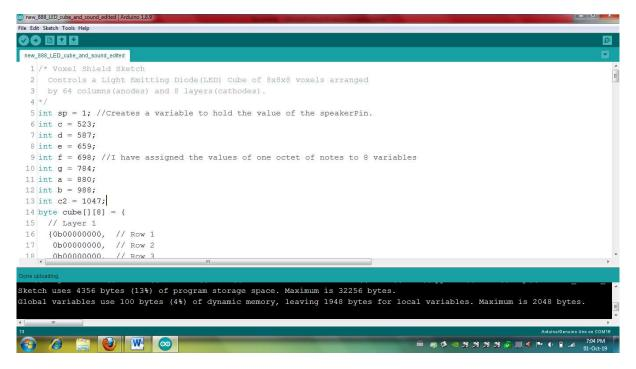
Figure 5 The photograph of the error free Arduino sketch showing .hex file after successfully verifying case
