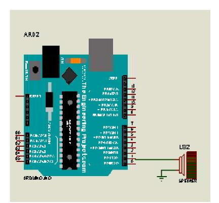
Figure 2 Circuit Diagram of Audio System
