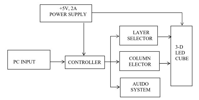
Figure 1 Block Diagram of Music Reactive LED Cube Control System
