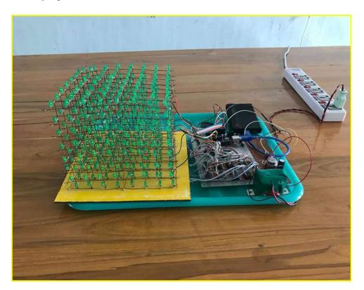
Figure 6 The photograph of the music reactive LED cube by Arduino Microcontroller
