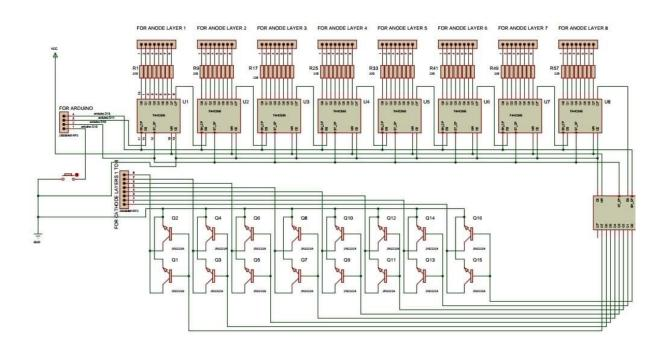
Figure 3 The circuit diagram of 8-column connection in 8×8×8 LED cube
